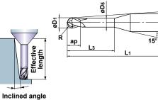
Ball nose end mill with PVD-coating for cobalt/chrome and titanium alloys
